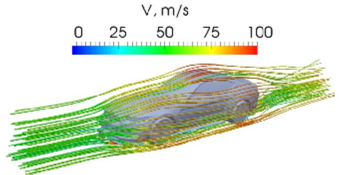
Simulation of an optimally dimpled Ford Mustang
