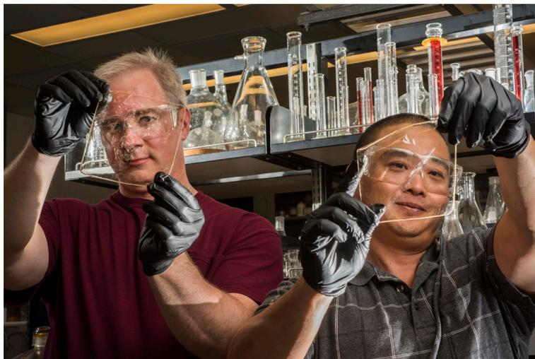
Sandia's membrane technology starts with a poly(phenylene) backbone that is chemically functionalized based on the intended application which greatly reduces manufacturing costs. For instance, the membrane can be optimized for transportation of protons (H<sup>+</sup>) or hydroxyl ions (OH<sup>-</sup>) depending on the acidic or alkaline environment of the energy-water system. To further reduce costs, the membrane is designed to eliminate the need for precious metal catalysts.
