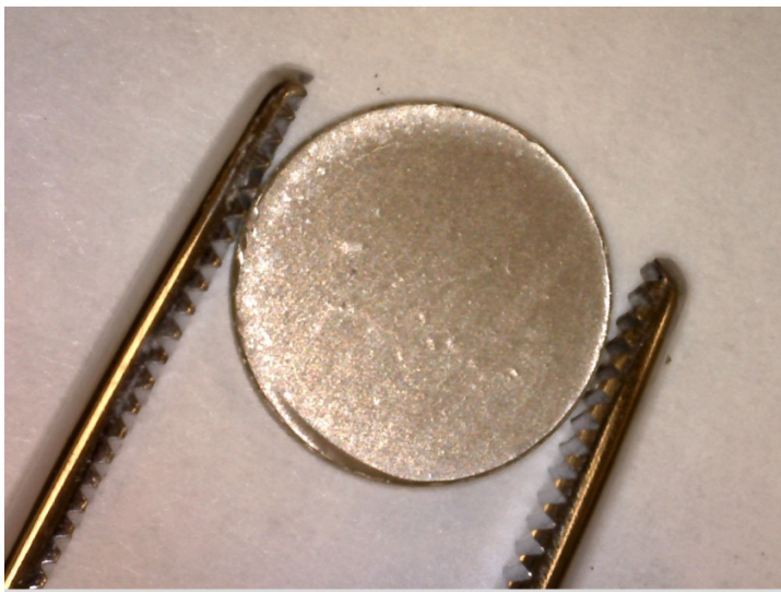
Tin matrix waste form mixed and pressed at 25,000 psi.
