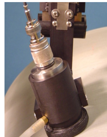
New probe holder allows for adjustable water path
